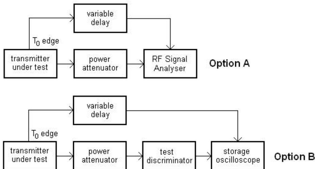
**Figure 6: Measurement arrangement for modulation accuracy**
